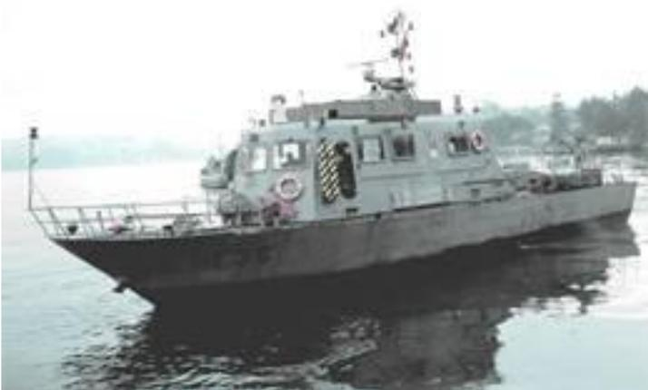
• **R/V Mesaha 2:** built in 1994; Length/Breadth: 21.28 mt/5.07 mt; Displacement: 47 ton Draft: 1.33 mt; Maximum Speed: 10 KTS; Endurance:400 mil; Main Engine 2 x 1000 HP; Accommodation: Crew 10 and Scientists 5.
