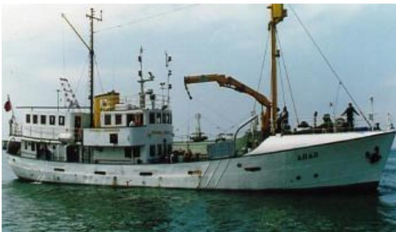
**R/V Avar:** Built in 1951; Length 31.27 m; Draft 3,20m; Tonnage 173,68 gross tons; Length 31.27; Draft (m) 2.76; Gross Tons 178.0; Capacity Dry Cargo Area (m<sup>3</sup>) 3.0; Fuel Capacity (m<sup>3</sup>) 30.0; Area Wetlab (m<sup>2</sup>) 8.0; Area Drylab (m<sup>2</sup>) 10.0; Free Deck Area (m<sup>2</sup>) 55.0; Range (n mi) 5000.0; Speed Cruise (kt) 9.0; Speed Max (kt) 11.0; Endurance (days) 30.0; Accommodation - Officers 2, Crew 11, Scientists 15; Air
